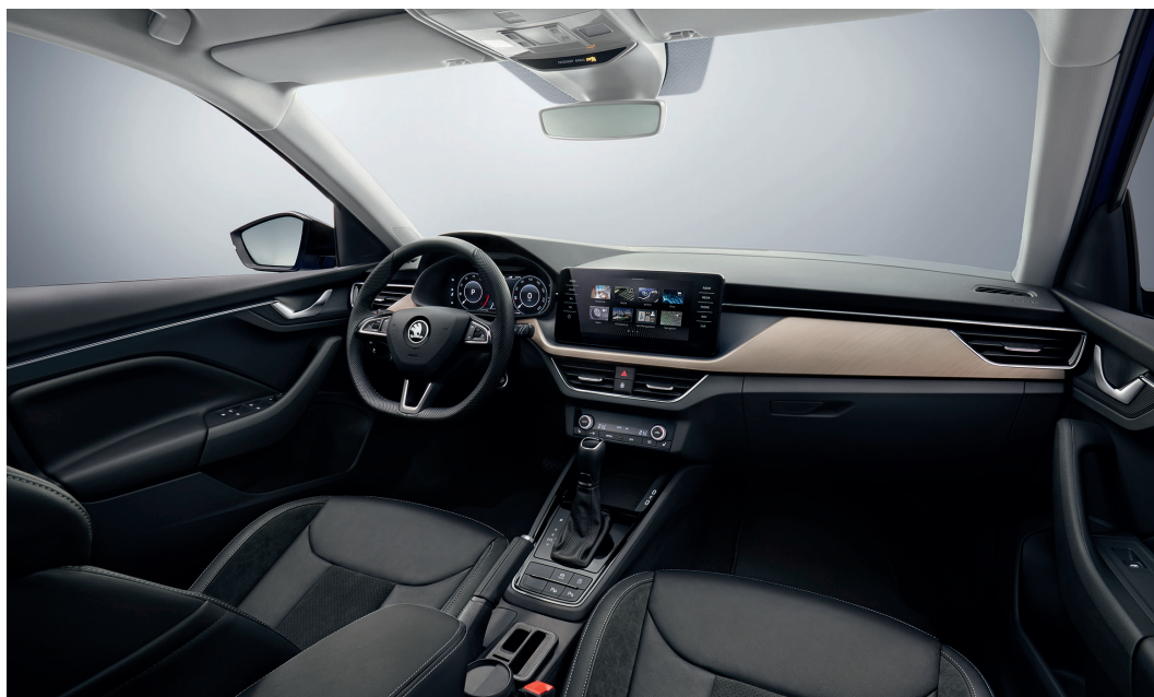
Fig. 1. PP compound Daplen EE001AI has good scratch resistance and surface quality despite its low material density of 0.95 \text{ g/cm}^3 . Skoda therefore relies on this material for the door trim of its Scaa (© Skoda)
